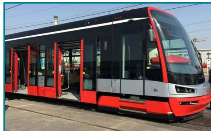
CRRC Qingdao Sifang fuel cell tram demonstration in 2015, powered by Ballard
