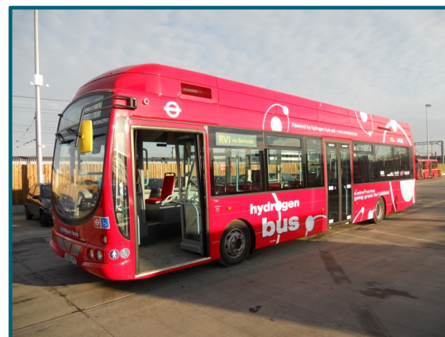
One of eight fuel cell buses in TfL's London, U.K. fleet, powered by Ballard
