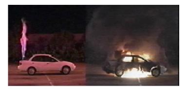
Photo from a video that compares fires from an intentionally ignited hydrogen tank release to a small gasoline fuel line leak.
