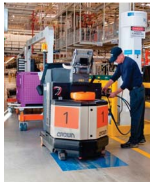
ABOVE: BMW employee pumps hydrogen into the forklift's fuel cell power pack.
