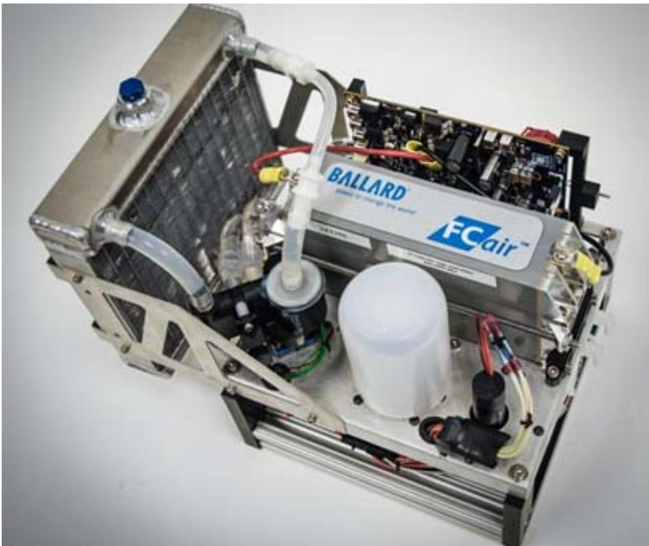
Ballard FCair® -600 fuel cell system for powering UAVs or drones. Source: [www.ballard.com](http://www.ballard.com)
